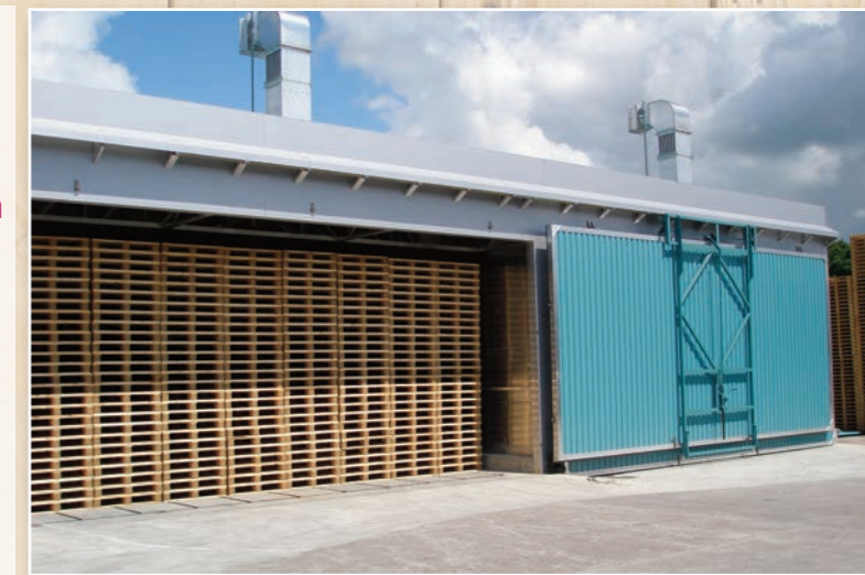
2 Kilns each holding 1225 Euro pallets
