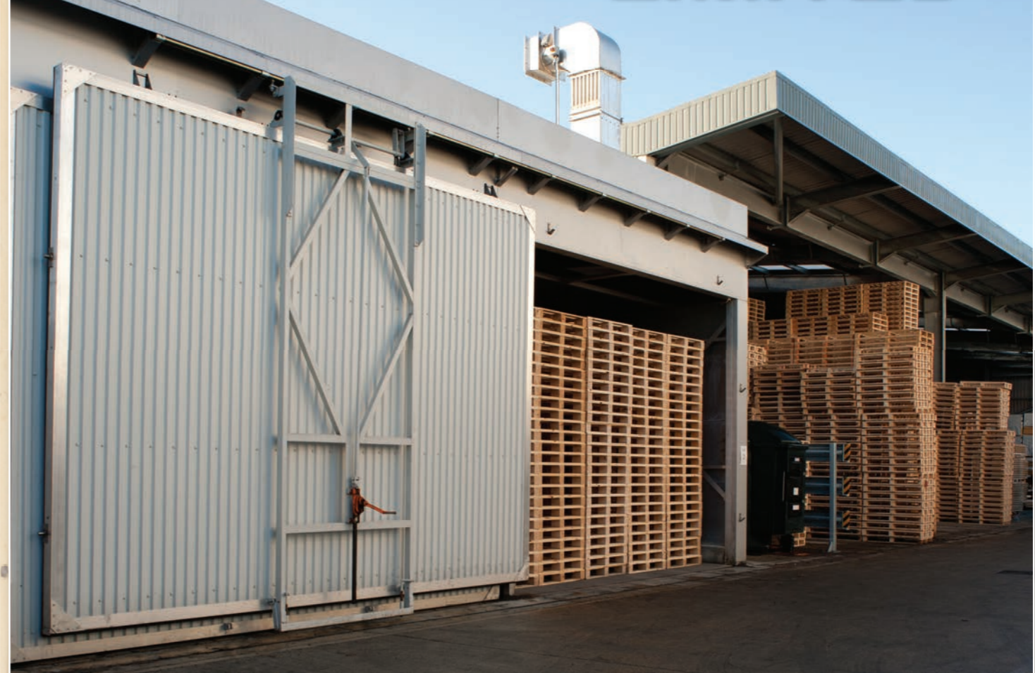
2 kilns with the capacity of 700 Euro pallets each
