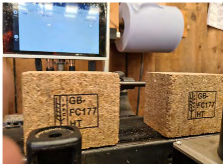
Printing pallet blocks on a conveyor using a piezo inkjet printer
