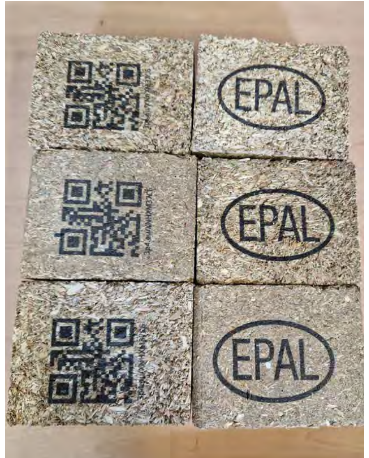
Composite blocks marked with the EPAL logo and scannable QR code using inkjet printing
