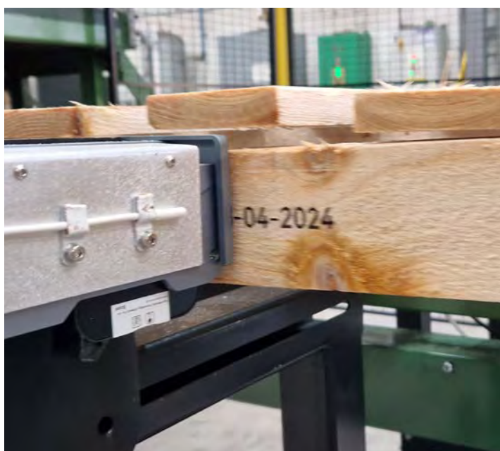
Printing a two-way pallet bearer 25mm high using thermal inkjet
